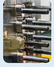
Z-420 PM® SuperMelt Powdered Metal stainless mold material is a terrific choice for long run or high production molds where high wear resistance combined with corrosion resistance are required.
