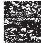
The uniform distribution of carbides in the powder- metallurgical structure compared to conventional tool steels with big carbides and carbide clusters.
